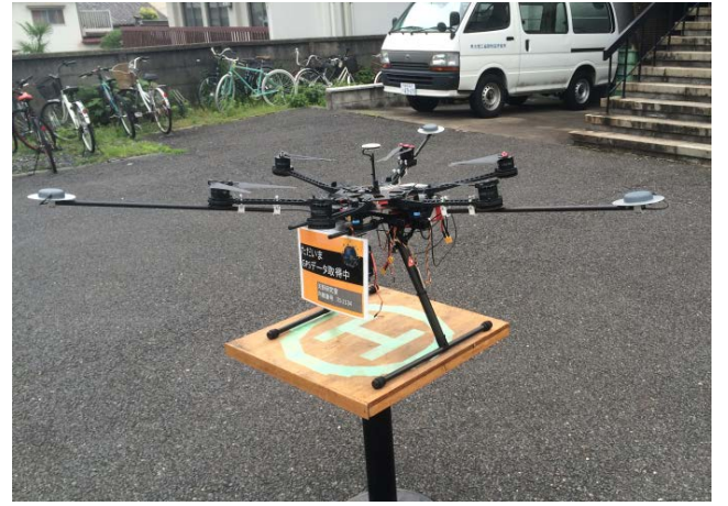
Fig. 10 Test environment for position and attitude determination in the static test.
