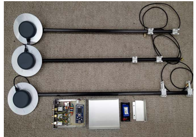
Fig. 3 Prototype multiple-GNSS data logging system.
