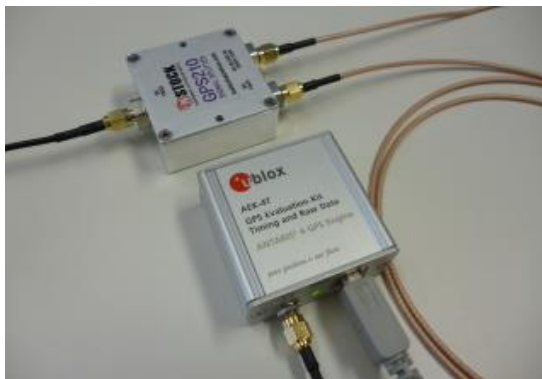
Using GPS signal splitter and another GPS receiver
