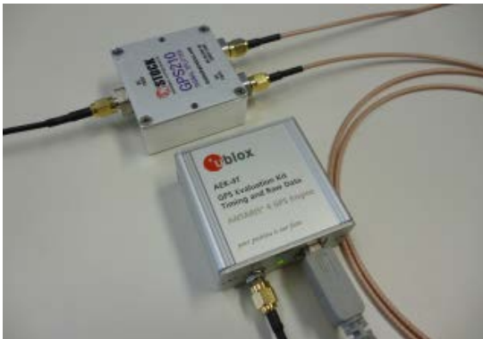
Using GPS signal splitter and another GPS receiver ( http://blog.goo.ne.jp/osqzss )
