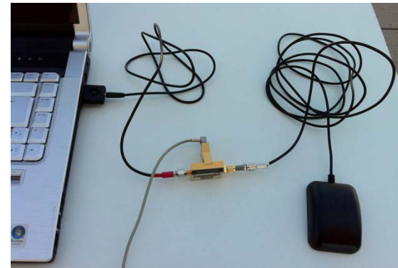
Using a bias-T network ( http://gnss-sdr.org )
